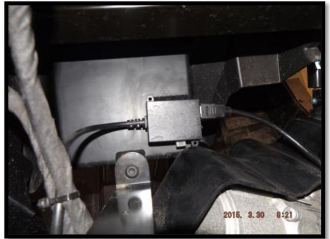
7. Zip tie or fasten excess cable to the wiring harness to prevent possibility of damage during use.
