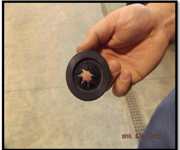
5. Route diagnostic cable through the grommet and into the dash of the RZR 900. Replace the grommet into the original location. The diagnostic plug will now be located under the dash.
