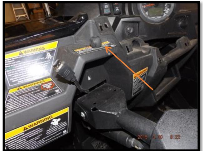
9. Assemble the mount and place the Bully Dog GT Tuner on the mount. Connect the USB cable into the Bully Dog GT Tuner.
