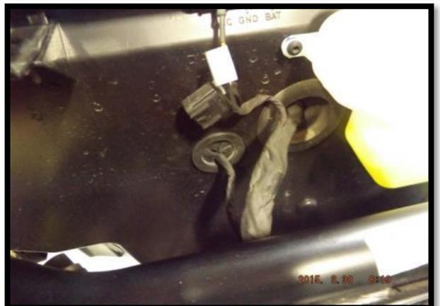
6. Velcro the Bully Dog GT Diagnostic Module Connector to the inside of the RZR 900 dashboard. Connect the '15 RZR 900 diagnostic connector to the Bully Dog GT Diagnostic Module Connector. Ensure the Module is set in the battery position (should come in this setting).
