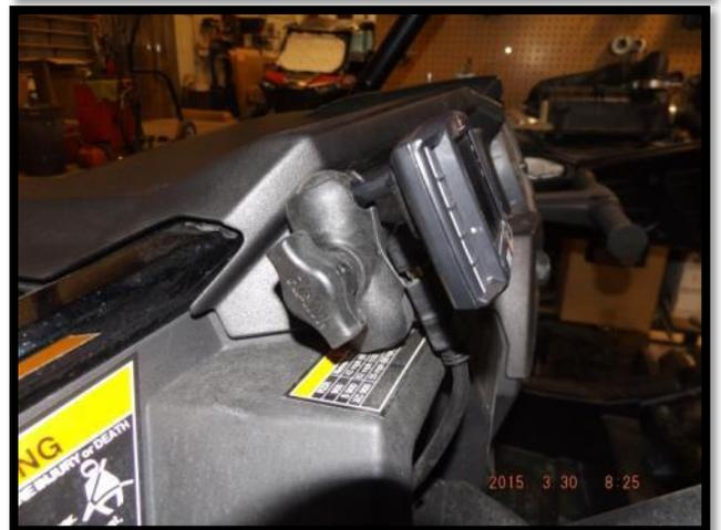
10. Bully Dog GT Tuner should be visible through the steering wheel as shown here.
