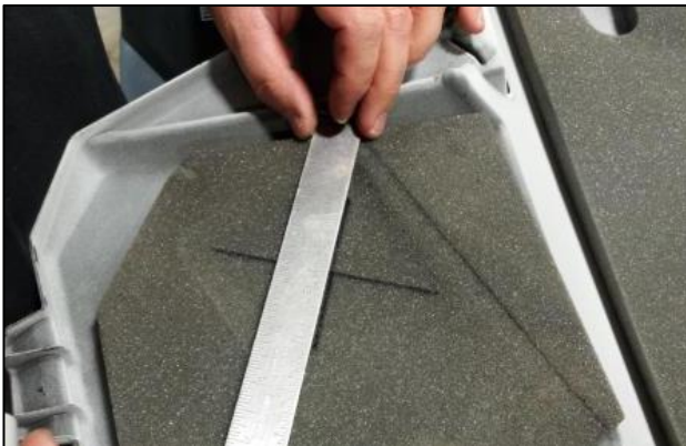
9. Using a straight edge, draw a line from corner to corner within the imprint shown.
