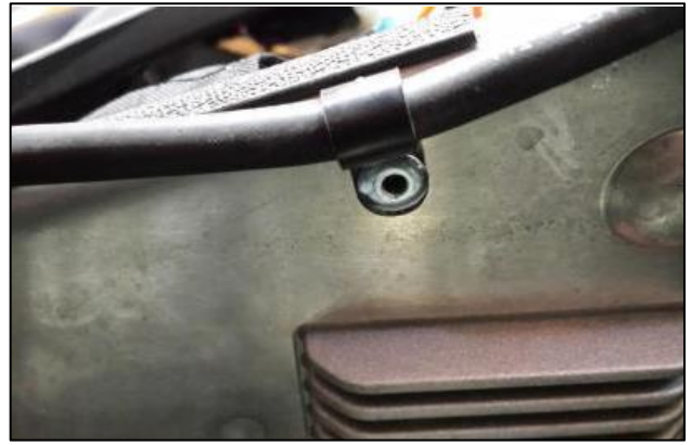
6. Place wire holder onto the Blow Hole wire then rivet into place as shown.
