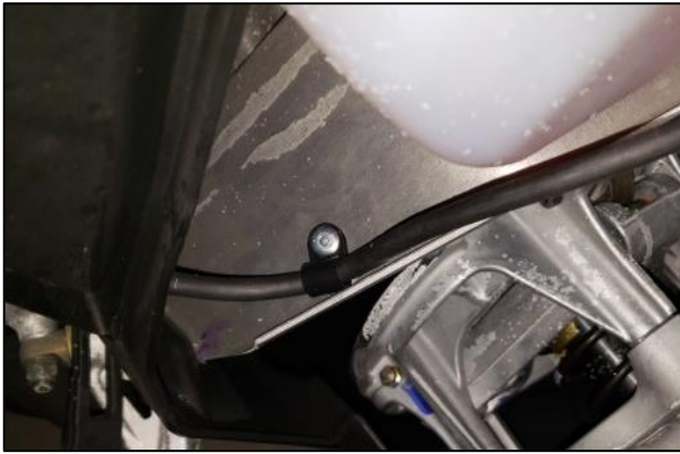
5. Drill a 3/16" hole in the aluminum shelf measuring 3" back from the front of the shelf.
