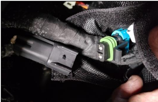
7. Route harness up the frame to harness bag under the center console. Locate plug cap labeled RCA ACCY POWER . Remove cap and plug Blow Hole into Accy Plug as shown.
