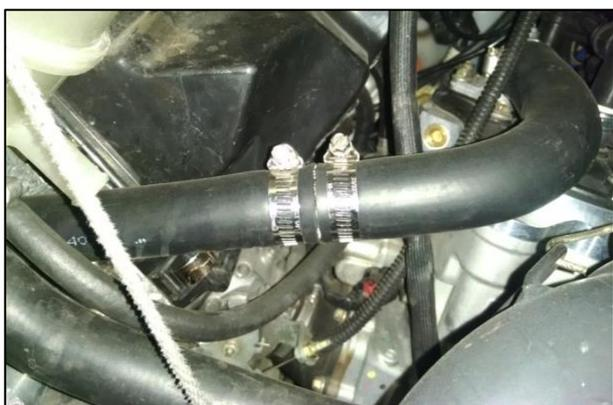
7. ('11-'15 ONLY) Insert splice and tighten hose clamps. Rotate and install onto the right hand cooler fitting with clamp. Secure with Zip Ties
