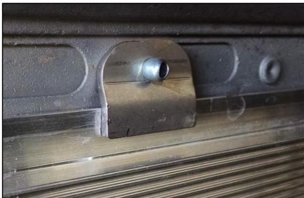
5. Secure the cooler with one rivet in the front and back. Align remaining rivets and secure. Rivet clamp plates under the tunnel as shown.
