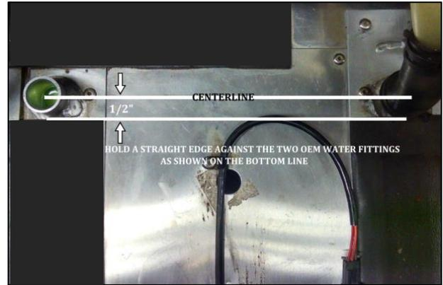
2. Use a straight edge to mark the OEM cooler fittings as shown. Measure up 1/2" and mark on both sides of the tunnel. Cut out attached template and lay between the OEM cooler extrusions. Center punch on each center marks.
