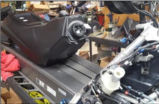
1. Remove rear suspension, track, seat, and fuel tank. Driveshaft & track removal not required but recommended. Remove left hand cooler hose and drain the cooling system. A clean shop vacuum set up for liquid works best.
