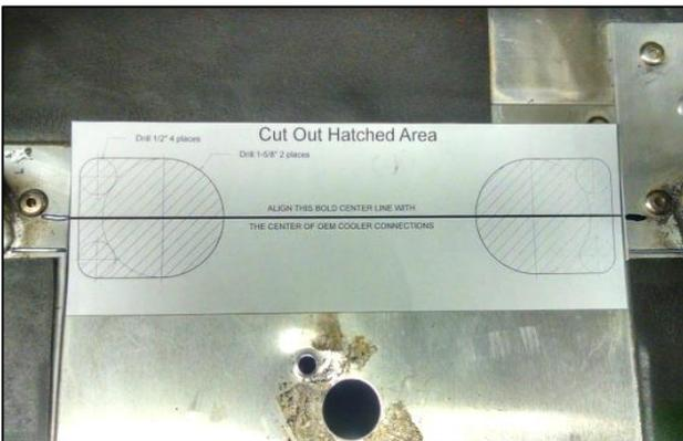
3. Drill a small pilot hole first then using an 1 7/8" hole saw, drill out the larger hole. Clean all shavings and rivet mandrels before continuing.
