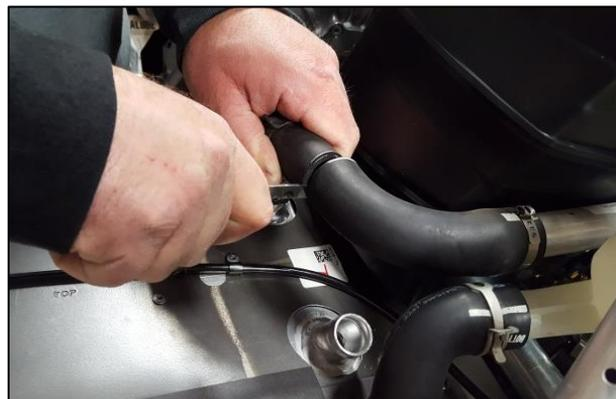
6. Use the Hose Cut Guide to cut the hose which comes off the cylinder head thermostat. Install and secure with hose clamps. ('11-'15 SEE STEP 7)
