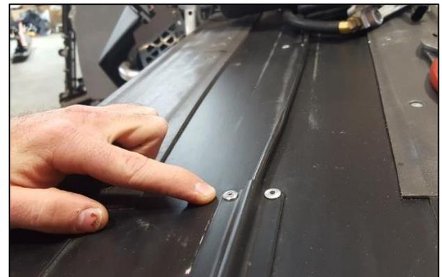
4. Use the taillight wire guide to mark new locations for the rivets down the center. This will ensure correct location. Make sure the front is centered in the tunnel before marking. Insert Tunnel Cooler through the drilled holes.
