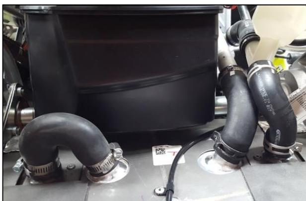
8. Install 180° hose and clamps with the long leg on the new cooler fitting. Make sure clamps are tight. Reinstall gas tank, seat, and track.
