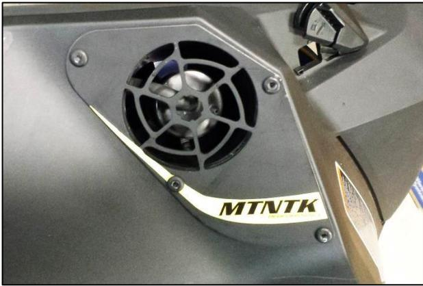
5. Remove foam from inside of your panel. Rivet Blow Hole in place with 3/16" expanding rivets.
