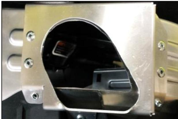
9. Using bracket as a guide, only cut aluminum clutch cover as shown. De-bur everything when finished cutting. Plug the Blow Hole into
