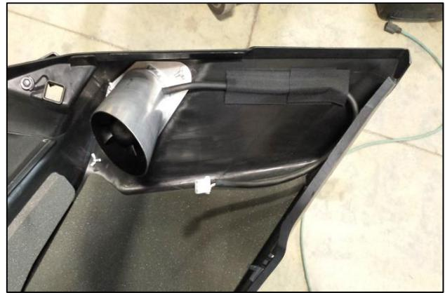
6. Clean entire surface and install hook & loop fastener to keep wire in proper place on panel.
