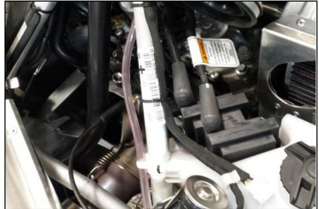
2. Route extension harness down and over the structure tube and onto the top of oil tank. Replace the hood and gauge console. Reconnect the headlights, gauge console and air-temp connectors back together.
