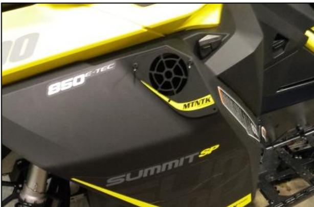
3. Hold face plate up to PTO side panel. Align top and back corner edges as shown. Using a silver marker or pen, mark holes to be drilled. Drill out the marked 3/16" holes & Insert rivets one at a time to hold face plate in place.
