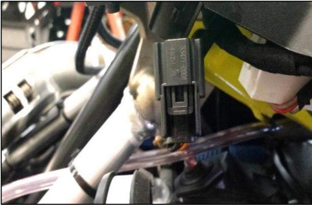
1. Remove side panels, gauge console, hood, and glove compartment cover. Find connection site on the left-hand side near the hand warmer switch under the console. Route Blow Hole extension harness to the connection port.
