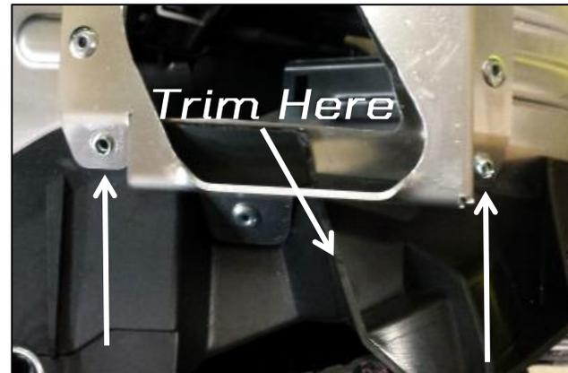
8. You will have to trim the plastic cover as shown. Install remaining 6 rivets with 2 being installed from the inside-out as shown.
