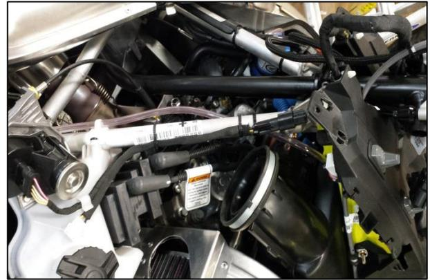
2. Route extension harness down and over the structure tube and onto the top of oil tank. Replace the hood and gauge console. Reconnect the headlights, gauge console and air-temp connectors back together.
