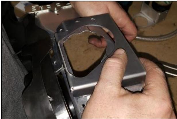
7. Slip the Bracket in-between the aluminum clutch cover and the black shroud. Align bracket with hole of large head rivet previously drilled. Mark holes to be drilled out.
