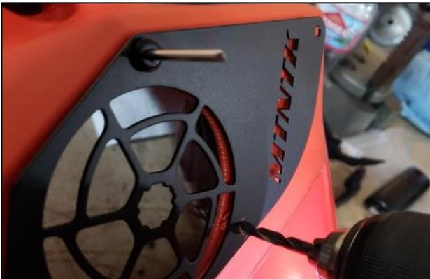
3. Hold face plate up to PTO side panel. Align top and back corner edges as shown. Using a silver marker or pen, mark holes to be drilled. Drill out the marked 3/16" holes. Insert rivets one at a time to hold face plate in place.
