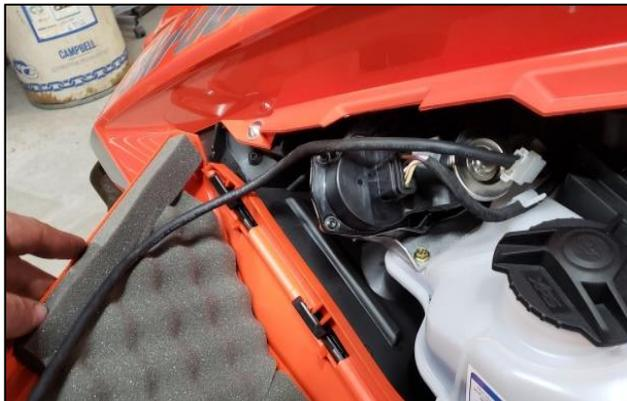
9. Route Blow Hole wire away from clutches and plug into white harness connector.
