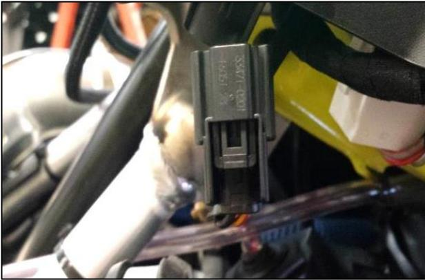
1. Remove side panels, gauge console, hood, and the glove compartment. Find the accessory plug connection site on the PTO side and route the Blow Hole extension harness to the Factory Accessory plug
