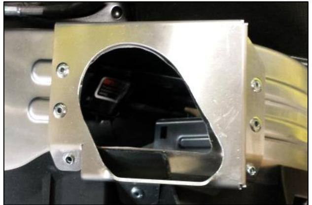
8. Using bracket as a guide cut aluminum clutch cover as shown. Install remaining 6 rivets with 2 being installed from the inside-out as shown.
