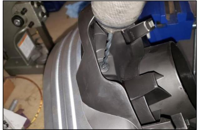
6. Remove clutch cover from machine. Drill out the large head rivet on plastic shroud as shown.
