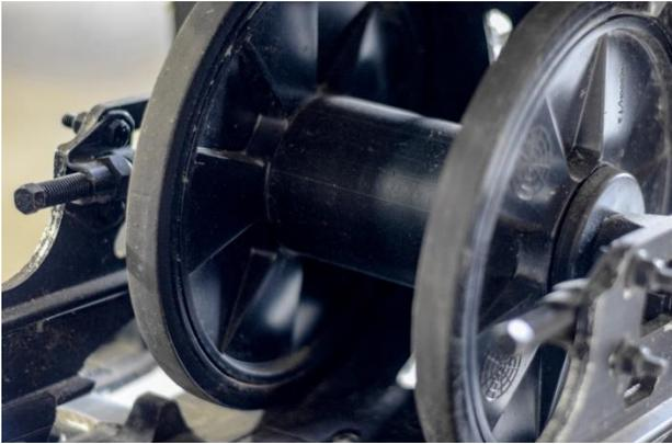
1. Remove the stock rear wheels by loosening the track adjustments bolts and remove the rear axle bolt. Remove the plastic center collar and discard. Remove track adjustment blocks and drill the adjustment collar hole out to  $\frac{3}{8}$ "
