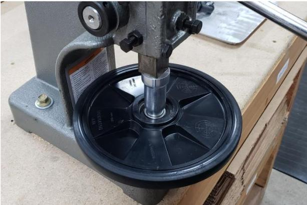
3. Use a press to install standoff assembly onto the stock rear wheel as shown. Be sure standoff is on the snap ring side. Press bearing to shoulder.
