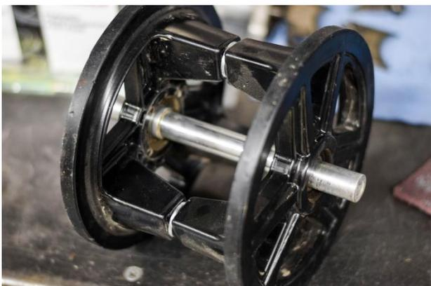
5. Bolt second Tough Wheel onto stock axle as shown. Tighten connector bolts. Install Tough Wheels into rear skid in stock location. Align track adjustment collars with skid windows.
