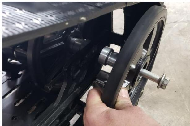
6. Bolt outer wheel into axle as shown. Be sure the standoff is toward the inside of the wheel and the bolt is directly against the wheel. Apply Loctite and leave bolts loose till track is aligned.
