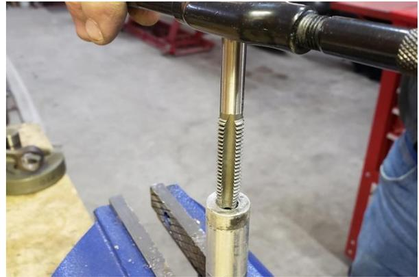
2. Using a M12x1.75 Tap, carefully tap the stock rear axle as shown. Make sure to do this carefully. Once finished, remove all burs and shavings from shaft.
