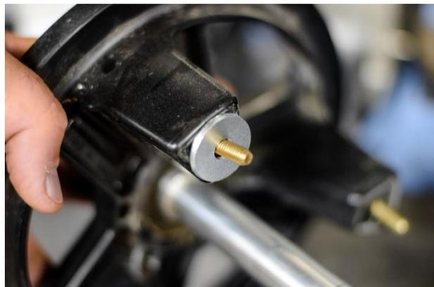
4. Install the stock axle onto the new Tough Wheel. Install the three wheel connector bolts and spacers onto connector bolt as shown.
